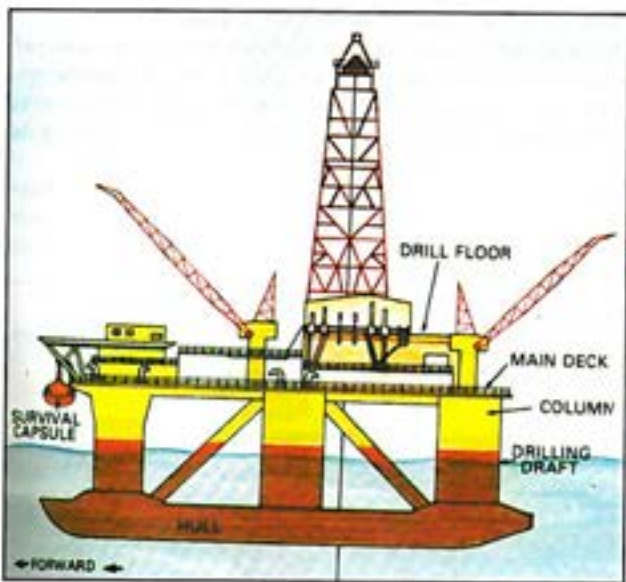
Fig. 3- A column-stabilized semi submersible rests below the waterline when in the drilling mode.
