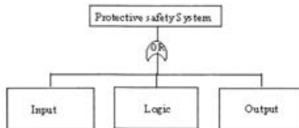
Fig-7: Fault tree of Protective Safety Systems
