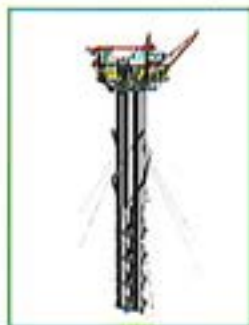
Figure 2: Schematic of a Cell Spar Lately, with more competition in the market and the desire to drive costs
